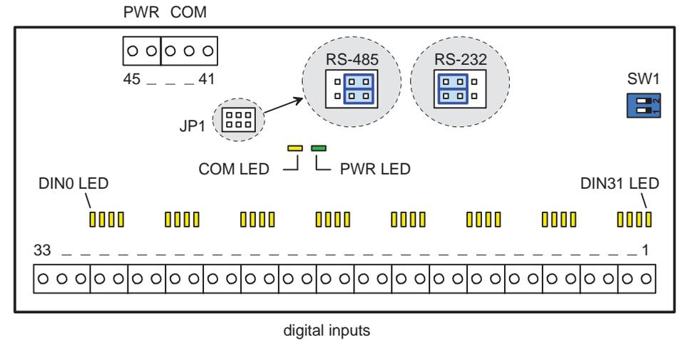
*Note: The figure shows LEDs indicating the presence of supply voltage, the activity of the communication line and the presence of voltage at the inputs (only when the power supply is on). Two plug-in jumpers are intended for the configuration of the communication line type*
