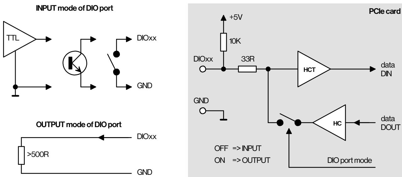
**Figure 3.** Simplified schematic of DIO ports.
