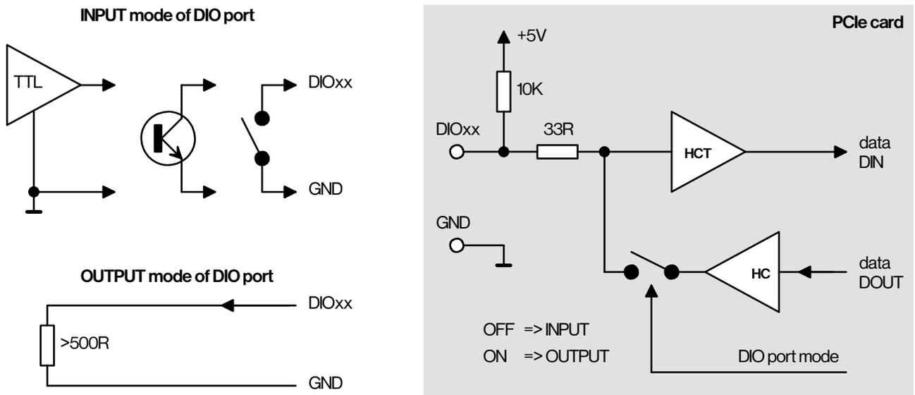
Figure 3. Simplified schematic of DIO ports.
