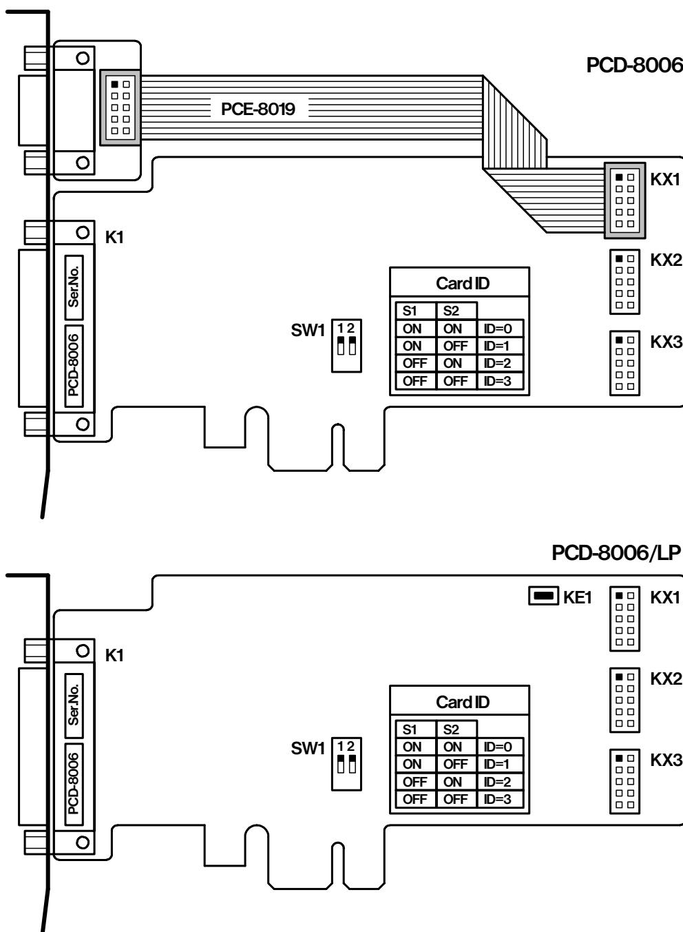
**Figure 1.** Location of switches and connectors on both version of card.
