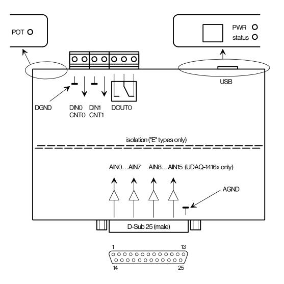
Figure 2. Location of important points on UDAQ-1408CA/CE/DA/DE and UDAQ-1416CA/CE module (top view).
