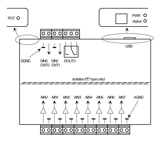
Figure 1. Location of important points on UDAQ-1408A/1408E module (top view).
